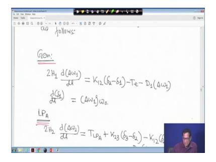
So, for the your what you call for therefore, for generator now we summarized this. Now, rewriting this equation for generator 2 H 1 d dt of delta omega 1 is equal to K 12 delta 2 minus delta 1 minus Te minus D 1 delta omega 1. Now, d dt of delta 1 delta omega 1 into omega 0.
