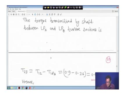
The torque transmitted by the shaft between LP A and LP B turbine section will be similarly that your T 23 will be T 12 minus T LP A, right is equal to this much minus 0.216 it will be 0.684 per unit, right. The hence your delta 32 will be delta 3 minus delta 2 is equal to T 23 upon K 23. So, T 23 is known, K 23 also you have computed before, so it will become 0.02185 electrical radian. Although this variation if you look it is very small, but it has some meaning, right.
