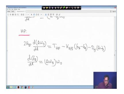
Now, for high pressure this section 5. It is 2 H 5 d dt of delta omega 5 is equal to T HP that are the input torque minus K 45 into delta 5 minus delta 4 minus D 5 delta omega 5. This is for the high pressure portion, section 5. And d dt of delta 5 will be delta omega 5 omega 0. This is how we have to represent that each section, right.
