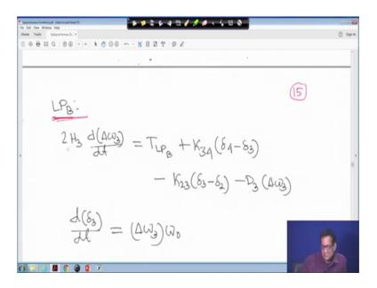
Similarly, for section 3 same way you will write 2 H 3 which will be d dt of delta omega 3 is equal to this is the input torque, right that it T LP B that is that is the section b that low pressure turbine, right. T LP B plus K 3 4 into delta 4 minus delta 3 minus K 23
