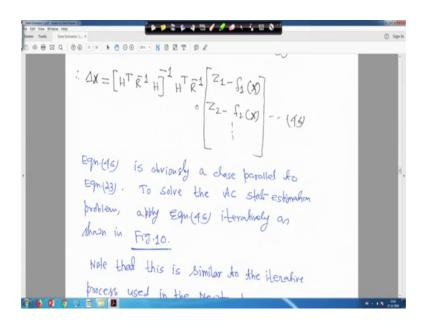
So, ultimately it will become delta x is equal to H transpose R inverse H whole inverse H transpose R inverse, Z 1 minus f 1 x Z 2 minus f 2 x this is equation 46 right. So, equation 46 is; obviously, close parallel to equation 23, because if you look equation 23 you will find very close to that right. To solve the ac state estimation problem you apply equation 46 iteratively as shown in figure 10 that means, a flow chart is given right.
