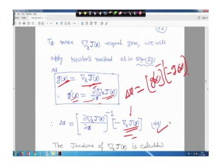
Now, to make this gradient 0 right we will apply Newton method as given in equation 37 right. So, in equation 37 actually this is actually assume that your gx is equal to; gx is equal to gradient of J x right therefore, g; that means, g dash x will be del x of gradient of J x, because J because you have to; you have to solve it iteratively right.
