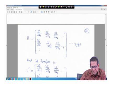
That means; that means, this H can be written as delta f 1 delta x 1, delta f 1 delta x 2 delta f 1 delta x 3 and so on up to nm number of your what you call measurement you have right. Similarly, delta f 2 upon delta x 1, delta f 2 upon delta x 2, delta f 2 upon delta x 3 and so on right.
