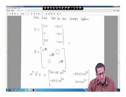
In this case the H transpose R inverse H matrix using the standard least square method would look like this for the sample system sorry. So, H was given the same H was taken
