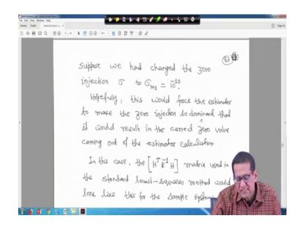
Suppose we had a change the 0 injection sigma for that is sigma M 1 is 10 to the power minus 10; that means, the meter is actually very accurate 10 to the power minus 10 sigma means, it is almost 0 error right suppose you have made it. Hopefully this would force the estimator to make the 0 injection. So, dominant that it would result in the your correct 0 value, coming out of the estimator calculator right.
