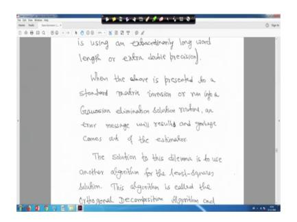
So, when the above is presented to a standard matrix inversion or run into a Gaussian elimination solution routine right and error message will result and garbage comes out of the estimator, because you will not get anything because matrix becoming singular.
