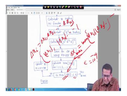
So, calculate now H transpose R inverse H matrix right so, that you can calculate. Now calculate H transpose R inverse H inverse now you have to calculate this one right step by step. Then you solve for delta x using equation 46, that this equation that is your this using this equation you solve for delta that is delta x 1, delta x 2 like this it is in general is what you call is a vector right.
