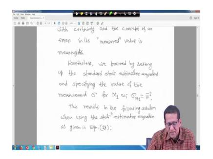
Now, nonetheless we proceed by setting of the standard state estimator right equations and specifying the value of the measurement sigma for M 1. Suppose for M 1 that sigma M 1 that is a standard deviation is 10 to the power minus 2 per meter 1 which was corrected near bus 1 right this result in the following solution when using the state estimated equation 33.
