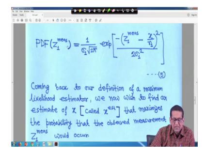
That your this term that Z 1, Z true that is your Z true it will be x upon r, because Z is the ampere your ammeter reading say, it is ampere and x is the volt, so volt by your resistance r so ampere. So, Z actually, Z true is actually x upon r 1, this term is replaced by x upon r 1. That means, by PDF Z 1 measure is equal to 1 upon sigma 1 root over 2 pi e to the power minus bracket Z 1 measure minus x upon r 1 whole square upon 2 sigma 1 square this is equation 5 right.
