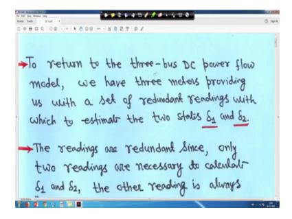
So, now to return to the three-bus DC power flow model, we have three meters providing us with a set of redundant readings with which to estimate the two states that is delta 1 and delta 2. There are two states, but we had three measurements right.
