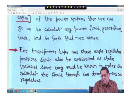
The transformer taps and phase angle regulator positions should also be considered as state variable since they must be known in order to calculate the flows through the transformers on and regulators right. So, that is what we have seen. Now just hold on. Let me increase the size.
