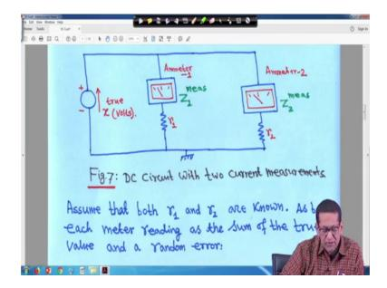
Now, suppose now I have now we have say two ammeters, pay in parallel and one resistance is r 1 here one resistance is r 2 here, current measure by ammeter-1 is Z 1 measure and current measured by your ammeter-2 it is your Z 2 measure right. And this is the true value of the voltage that is v. We have to estimate that true value, and this ammeter has standard deviation sigma 1 and this ammeter has standard deviation sigma 2 right.
