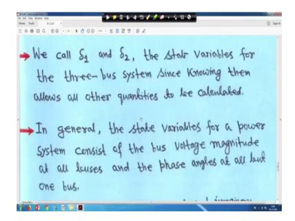
So, in general the state variables for a power system consists of the bus voltage magnitude at all buses and the phase angle at all but one bus that is slag bus right.
