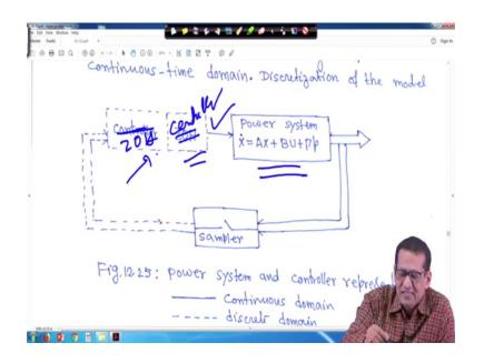
So, this block diagram I told you that power system is in continuous time domain and controller is always in your discrete domain right and this is the sampler and this controller is there 0 order hold is there. So, I told you that ah whenever you will solve I mean I mean nowadays you are putting in the matlab and getting the result, but my suggestion is that if you write the code of your own you have to follow this logic.
