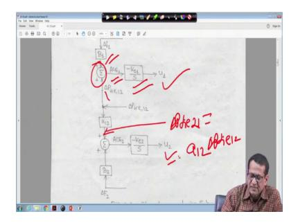
So, in that case just hold on little bit little bit ok. So, this one in the second case your this is minus this is minus K I integral controller. So, this is B 1 delta f 1 and this is the structure of the integral controller. And delta P tie 1 2 is coming these two are added and this is that area control error 1 and this is output U 1 right. That I told you initially U 1 is equal to integral of minus K I 1 integral of a c 1 D t.
