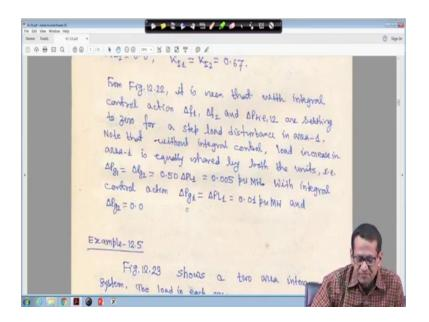
So, that is why that is why this figure 2 2 what I showed that it is seen that with the integral control action delta f 1 delta f 2 and delta P tie 1 2 are settling to 0 for a step load disturbance in area 1. Note that without integral control load increase in area 1 is equally shared by both the units that is delta P g 1 is equal to delta P g 2 is equal to 0.5 P L or half of P L 1.
