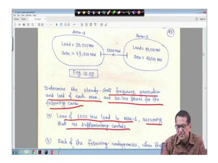
So, we have to so we have to these are these are given these are the area 1 area 2 every everything is given right. So, load here is 2000 megawatt and load 4000 megawatt and generation this side is given. So, determine the steady state frequency generation and load each area and tie line power for the following cases. Loss of 1000 megawatt load in area 1 assuming that no supplementary controls right. So, this is one and another one.
