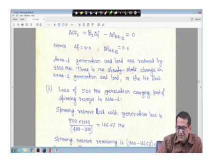
Hence delta f is equal to 0 and delta P tie 1 2 is 0 right. So, area 1 generation and load are reduced by 1000 megawatt. So, there is no steady state change in area 2 generation and load or the tie flow right. Now, loss of 500 megawatt generation carrying part spinning reserve in area 1.
