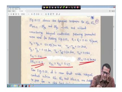
And we have taken equal area capacities. So, a 1 2 is minus 1, there is no load disturbance in area 2. So, delta P L 2 is equal to your 0 and integral gain setting. We have taken K I 1 is equal to K I 2 is equal to 0.76 and load disturbance in area 1 we have taken delta PL1 is equal to 0.01 per unit megawatt right.
