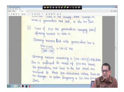
So, spinning reserve lost with generation loss is it will be simply 1000 by 4000 minus 1000 into 500 so 166.67 megawatt right simply arithmetic. So, spinning reserve meaning is 1000 minus 166.67 so 833.33 megawatt. This is sufficient to make up 500 megawatt. Hence the generation and load in the two areas are restored to their pre disturbance values.
