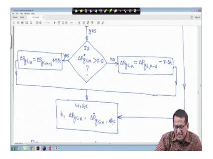
So, next is that we are checking that absolute of delta P g i k greater than r or not right. First we have to check if it is no then directly you will go, but if it is yes then you check whether it is greater than 0 or not. If it is a positive then this side left hand side is delta P g i k is equal to delta P g i k minus 1 plus r into delta t. So, it moves like a straight line because of r into delta T plus this one.
