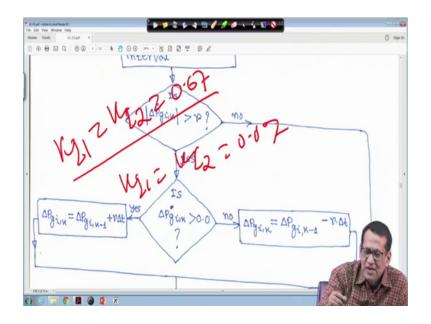
Whatever simulation I have shown you that K I 1 is equal to K I 2 we have taken 0.67 this is without generation rate constant right. But in reality this generation arte constants are there for any thermal unit. So, in that case the integral gain should be very small for example, K I 1 will be is equal to K I 2 say is equal to 0.07 or even less right. So, it is a very small otherwise what will happen your system will become unstable for higher gain.
