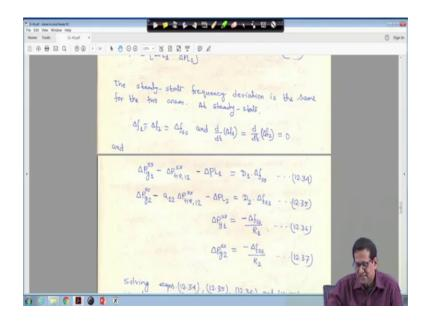
If it is so, then this equation we can write delta P g1 steady state minus delta P tie 12 steady state minus delta p L1 is equal to D 1 into delta f s s. If delta P tie 12 ss from right hand side, it has brought to the left hand side. So, this is equation- 34.
