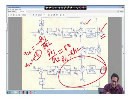
Just suppose a 12 is equal to minus P r 1 upon say P r 2 right. Now, suppose my P r1 upon P r2 is equal to say 8.0 right. This is the ratio this is the ratio that means, that means, my a 12 is equal to minus 8 that means P r 1 is equal to 8 times P r 2 that means, if P r 1 is 100 megawatt sorry P r 2 is 100 megawatt, then P r 1 will be your 800 megawatt.
