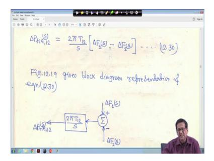
So, therefore this is your this is your from the for this equation 30, this is the block diagram that delta P tie 12 s is equal to 2 pi T 12 upon s into delta F 1 s minus delta F 2 s, I mean this equation 30 right. Therefore, the total complete block diagram of two area system it is like this let me let me just reduce it is this thing just hold on.
