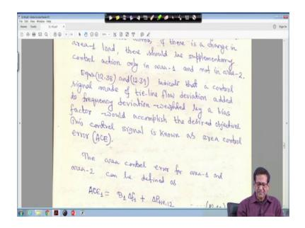
So, in other words if there is a change in area-1 load, there should be supplementary control action only in area-1 and not in area-2. Therefore, equation 38 and 39 indicate that a control signal made up tie line through deviation added to frequency deviation weighted by a bias factor that will see would accomplish that desired objective, this control signal in known as area control error. So, area control error basically it is a function of frequency deviation, and tie power deviation right.
