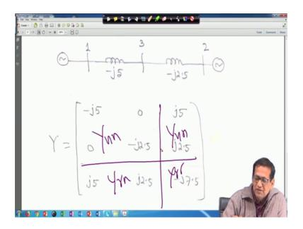
So, 1, 3 and 1, 2, 3, and it is easily you can compute the looking at this network, simply you can compute that your bus admittance matrix right. And your and again you will partition, because it is a 2 into 2 right it is a bus. And so this is your Y n n that is Y 2 into 2, this is Y n r, this is Y r n and this is Y r r right. And for following the same equation, you just go for matrix reduction.
