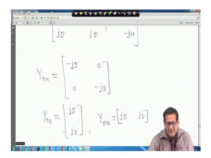
So, now you have to reduce it into 2 into 2 matrix. So, if we follow this using this so this is my Y n n I told you, and this is Y nr, and this is Y r n, and Y r r simply is a single element right, this is single element.
