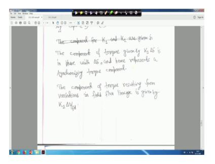
The component of torque given by K 1 delta delta I told you is in phase with delta. We will come to that later and hence represent a synchronizing torque component. The component of torque resulting from variation in field field flux linkage is given by K 2 delta psi fd right. The variations of delta psi psi fd is determined by the field circuit dynamic that is 3rd equation of 2 equation 267 right.
