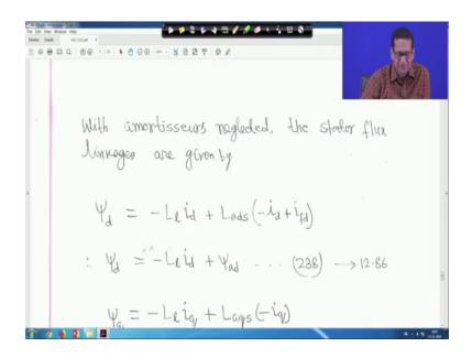
So, now, with amortisseurs neglected the stator flux linkage are given by t hat that go back to the stator circuit equation right this equation if I recall correctly go to the figure 28 right. So, from figure 28 that where analogous circuit is given flux then your inductance then your what you call that your current right. So, with amortisseurs neglected the stator flux linkage are given by this go to figure 20 which you have left out which we have left before right.
