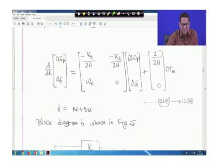
This equation can be written as x dot is equal to Ax plus Bu; that means, that means your x actually this is your a matrix right this is a matrix this is a 2 into 2 matrix right and this is your B and this is your u. So, actually u we are just we are representing like this u is equal to delta Tm right.
