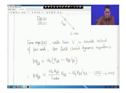
So, from equation 121 right this all these equations had been given before you go to equation 121 with time t in second instead of per unit the field circuit dynamic equation can be given as your p psi fd omega 0 efd minus Rfdifd from equation 121. I suggest that this all the lecture notes will be available to you just open it point of view because if I want to go back because of 121 much time will be lost right.
