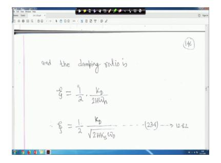
So, and the, that is and the psi is the damping ratio that is psi is equal to half into KD upon 2 H omega n right. So, therefore, the undamped natural frequency omega n is the this one right and your the damping ratio is psi is half into KD upon 2 H omega n. Now put omega n value and simplify you will get psi is equal to half KD root over 2 H KS omega 0 this is equation 234 forget about this one this is for my refer own reference.
