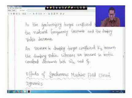
And increase in damping increasing damping torque coefficient KD increases the damping ration. Now KD is the new meritary if KD increases damping ratio increases right whereas, an increase in inertia constant decreases both omega n psi right. So, if it is in the your denominator H increases means psi will decrease right similarly here also it is in the root over KS omega 0 upon 2 H.
