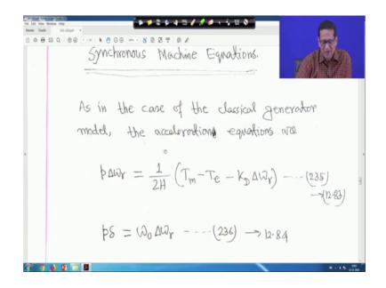
So, synchronous machine equations; this all that now and in the case of the classical generator model the accelerations equations are we have seen that p delta omega r is equal to 1 upon 2 H Tm minus Te minus KD delta omega r and p delta delta omega 0 delta omega r. Or in other ways small perturbation when you see p delta omega r upon 1 upon 2 H we have seen delta Tm minus delta Te minus KD delta omega r and p delta delta delta delta delta omega r ight.
