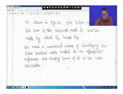
As shown in figure 26 the rotor angle delta is the sum of the internal angle delta i and the angle by which Et leads EB.
