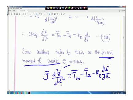
So, now some authors have written I mean many researches or authors they refer to 2H omega 0 as the per unit moment of inertia that is J bar is equal to 2H omega 0, because H you have seen from your stability studies that unit or dimension of H in second inertia is in second and omega 0 is radian per second.
