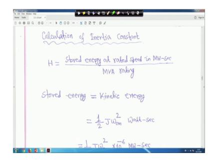
Now, calculation of inertia constant; so now we know from our power system studies, power system analysis transient stability studies are in machine that H is equal to store energy at rated speed in megawatt second divided by MVA rating right. So, its unit is second right. Therefore, stored energy is nothing but is equal to kinetic energy. So, we can write kinetic energy is equal to stored energy half J omega 0 m square that is watt second.
