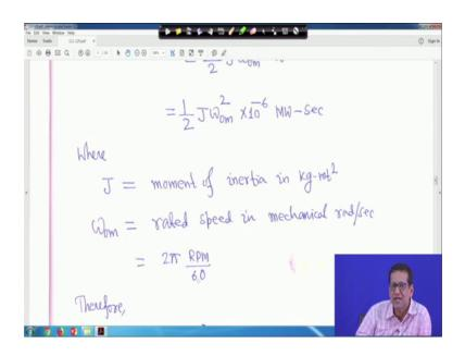
Where the energy is joule and we know joule per second is equal to watt. So, joule is equal to watt second. So, we write in watt second rather than joule right. So, we can write, now we if you convert watt into megawatt then it will be half J omega 0 m square into 10 to the power minus 6 megawatt second right because 10 to the power 6 watt is equal to 1 megawatt right.
