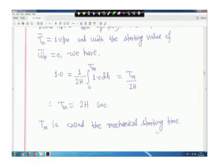
That means, we can write T m is equal to 2H second. So, T m is called the mechanical starting time. It is some rough, it is some approximate calculation. So, T m is called the mechanical starting time. So, it is 2H second because dimension are h is in second.
