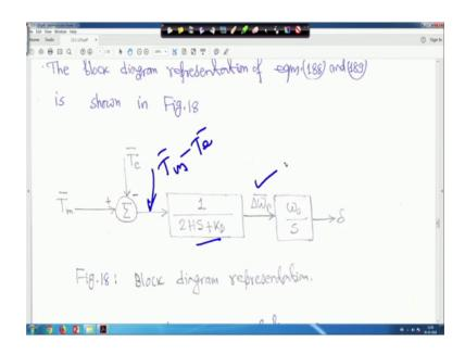
So, now the block diagram representation of equation 188. That means, this 2 equation and 189 is shown in figure 18 right.
