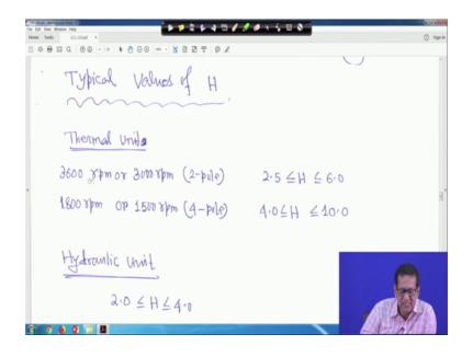
So, typical value of H; so generally for a machine that 3 6 3600 RPM or 3000 RPM right basically 2 pole machine for thermal power plant thermal unit is generally lies in between 2.5 and 6.0 second right. And if it is 1800 RPM or 1500 RPM that is 4 pole machines. So, it generally lies in between 4 and 10 second right. And similarly, for hydro unit hydraulic unit H is generally it by typical values lies in between 2 and 4 second right.
