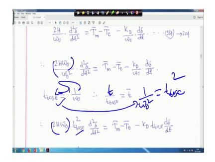
Now we know that earlier we have seen t base is nothing but 1 upon omega. So, it is 1 upon omega there is a time base right. Therefore, t by t base equal to t bar actually this is actually time it is actually t by t base is equal to t bar right time with if you take time in per unit and t base is equal to 1 upon omega 0.
