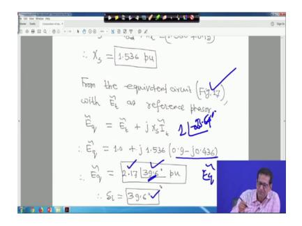
From the equivalent circuit just go back to figure 17 once, this figure 17 with E t tilde as reference phasor the simple single line circuit. if you see you see e q tilde is equal to E t tilde plus j X s into I 2 I t tilde right.
