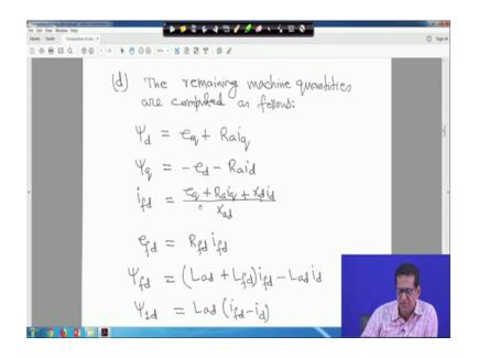
Therefore, the remaining machine quantities are computed as follows; therefore, already we have done this. Therefore, psi d will be e q plus Ra i q psi q will be minus e d minus Ra i d and this i f d expression also given before. So, i f d will be e q plus Ra i q plus X d i d upon X a d right. Therefore, and e f d there is a field voltage is equal to R f d into i f d. Equation numbers not given here because all these things are given before.
