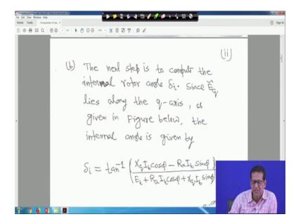
Now, this b part, the next step is to compute the internal rotor angle delta i. Since E q tilde lies along the key axis this we have seen earlier as given in figure below, the
