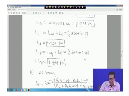
Similarly, L q is equal to L a q plus L l. So, it is 1.344, because here it is 1.344 we have computed plus 150.15. So, it is L q 1.4944unit.
