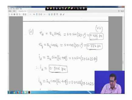
Now, part 2 e d we know e d is equal to E t sin delta i. So, E t is 1 and sin 39.1 degree that is 0.631 p u that is your e d. e q you know at E t cos delta i, so 1.0 cos 39.1 degree, So, 0.776 per unit that is my e q. And i d is equal to we know I t sin delta i plus phi. So, I t is 1 per unit delta i is 39.1 degree and phi is equal to 25.84 degree.
