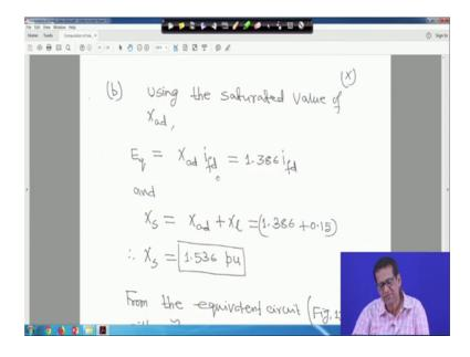
And part b using the saturated value of X a d we know that earlier we have seen e q is equal to J X a d i f d, but we are just thinking about the magnitude. Therefore, e q is equal to X a d into i f d that is 1.386 i f d right and X s will be X a d plus X l. So, X a d is 1.386 plus 0.15. That is X s is equal to 0.5536 per unit we call it as synchronous reactance right.
