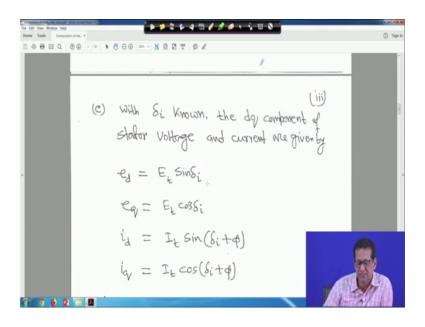
Now, with delta i known the d q component of stator voltage and current are given by this. We have seen earlier that e d is equal to E t sin delta i if delta i is known and e q is equal to E t cos delta i right. Similarly earlier we have seen that i d is equal to I t sin delta i plus phi and i q is equal to I t cos delta i plus phi. No, equation numbers given here because all these things we have seen in previous lecture right.
