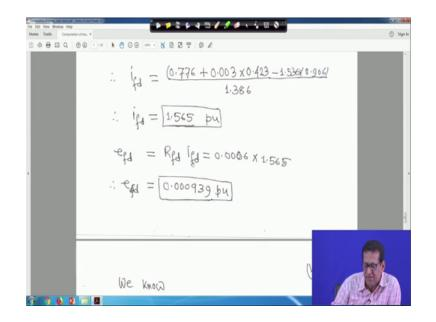
And we know e f d is equal to R f d into i f d. So, R f d is 0.666 into 1.565. So, e f d will be0.000939 per unit right.
