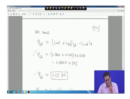
So, we also know that psi f d is equal to L a d plus L f d into i f d minus L a d into i a d i d right. So psi f d is equal to L a d 1.386 plus L f d 1.165 into i f d we have computed, 1.56 as minus. I told you L a d and X a d same right So, L a d is given 1.386 into i d 0.907. So, this comes psi f d 1.17 per unit right. We also know psi 1 d is equal to L a d i f d minus i d. So, psi 1 d will be 1.386 into in bracket i f d is 1.565 minus i d 0.909.
