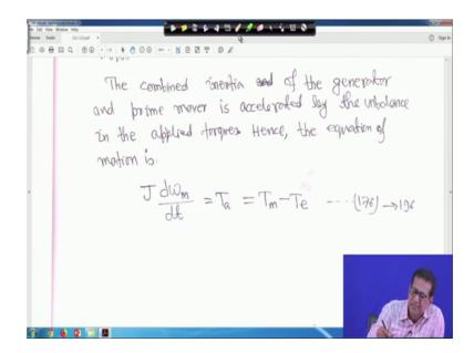
So, now the combine inertia of the generator and prime mover, prime mover means in power plant it is a turbine right. So, combine inertia of the generator and prime mover is accelerated by the unbalance in the applied torques. Hence, the equation of motion is given by J d omega m d t is equal to accelerating torque T a is equal to T m minus T e. This is equation 76 right. So, this one you should not read, this is equation 176 right.
