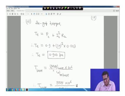
Now, number 3, the air gap torque, we know Te is equal to P t plus I t square r a. So, P t is 0.9 and I t is 1. So, 1 square and Ra is 0.003. So, basically it is coming t is equal to 0.903 per unit. If you neglect this loss then t approximately equal to P t because these are they are very close right. Now next is the torque base, the t base. Torque base is MVA base into 10 to the power 6 divided by omega mechanical base right.
