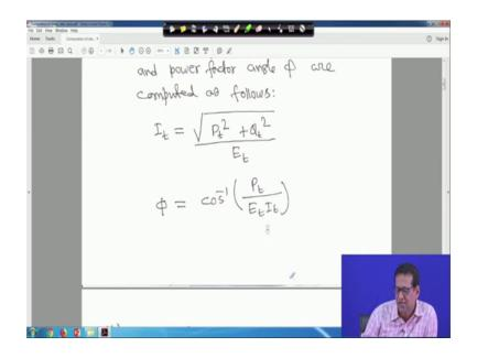
And similarly your power factor that cos phi will be P t upon E t, I t. E t is the magnitude, I t is the current. So, if P t is the real power and E t, I t is the volt ampere therefore, cos phi will be P t upon E t I t. Therefore, phi is equal to cos inverse P t upon E t I t right.
