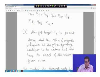
Part 3, that air gap torque Te in per unit in per unit newton meter right. Assume that the effect of magnetic saturation at the given operating condition is to reduce low your L a d. And L a q to 83.5 percent of the values given above that we will see when we solve this problem.
