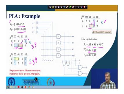
Now, if you want to realize a multiple logic function using PLA what will be the approach ok? So, we take example then it will be useful right. So, here is an example simple example for the sake of understanding. So, one function F 1 is getting generated is to be generated which has got min terms 2, 4, 5, 7 another one 0, 1, 2, 4, 6 ok.
