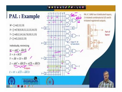
Now, if we have been given this you know PAL to realize it we see that for realizing W we need to generate two product term of four variables ok. So, four variables are fine that A naught to A 3 we name them as ABCD right, and corresponding this terms will be A A bar B B bar over here C C bar D D bar right this is there right and two product term we can generate like A, B, C prime. So, A is there connection we written B and C bar.
