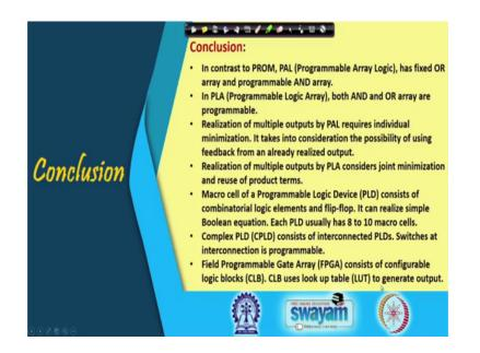
So, with this we conclude today's class, so what we have seen that in contrast to PROM PAL has fixed OR array and programmable AND array right and in PLA both and AND, OR array are programmable. And realization of multiple outputs by PAL requires individual minimization, it takes into consideration the possibility of using feedback from an already realized output and for PLA, we considered joint minimization and reuse of product terms ok.
