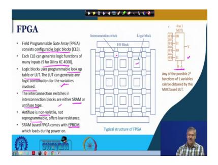
And when we talk about CPLD we should also talk about another such IC called family called FPGA ok. So, this field programmable gate array, so this is further you know advancement of CPLD, CPLD cannot provide much of a you know packing density and has got its limitations, so people have moved forward. So, these FPGAs consist of Configurable Logic Blocks or CLB ok. And each CLB can generate functions of many different inputs right each CLB ok.
