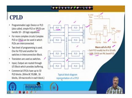
So, with this we go to what is called complex programmable logic device, so before that we just take a look at what we consider a macro cell of a programmable logic device ok. So, the way we had seen it before; the way we had seen before that there is a AND plane ok. So, from the AND plane this OR gate is taking the product terms alright this product term is going to a flip flop right. So, from this flip flop ok, so this flip flop we can see that we can select it to go to the next level ok.
