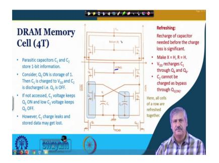
Now, we look at one DRAM memory cell, which is 4 transistor base; it is somewhat similar to what we had seen in case of 6 transistor base MOS based SRAM cell in the last class. So, there is some differences that we shall also tell.
