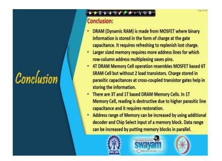
So, with this we come to the conclusion of this particular class. What we have seen? That dynamic RAM made from MOSFET stores charge, stores information in the form of charge which is available at the gate capacitance parasitic in nature because of the leakage it requires refreshing to replenish the lost charge. Larger size memory we can do better by multiplexed row column addressing which sets pins, number of pins that would be required for the memory IC.
