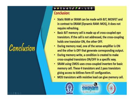
So, with this we conclude and what you have seen very quickly that static RAM or SRAM can be made with BJT, MOSFET, CMOS ok. And in each case we are looking at cross coupled inverters made up of transistors and their operating in bistable mode. And for BJT we have to seen how this sense amplifiers and write amplifiers work. Similarly, we had seen it the CMOS and normal MOS; so, the uses of pass transistors for reading and writing operation.
