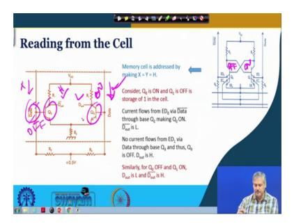
In contrast had been it been the case that this is ON and this is OFF ok, then current would have flown in this direction this is right ok. And it would not a flown in this direction because this is OFF so, this current is flowing in this so, this is will be ON and this will be OFF sorry not this one, this will be OFF right. So, this one will be high and this one will be low right.
