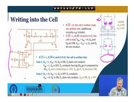
Now, we look at the writing operation ok. So, the circuit that you can see, now this is the basic memory cell ok. And generally we consider this is ON Q naught is ON and Q 1 is OFF right. And this is the data line or the bit line and this is the reading or sense amplifier.
