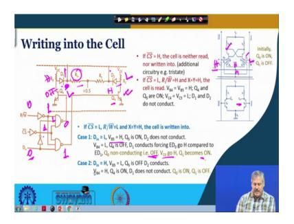
So, now, this read write bar input is 0 ok. So, this is 1 chip select is 0. So, this is 1 ok. Now, if D in is low. So, that is 0 ok. Then this is also 1 this is not gate. So, this is 1. So, this NAND gate output will be 0 and these NAND gate output will be 1, is it clear, this part is understood. Because of which this V B this particular base voltage of transistor Q 5 ok, this is high and this is low, what does it mean.
