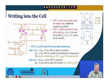
Then rest of the thing is if then this is high and this is high so, this 2 transistor Q 4 ON and Q 5 ON ok. So, this voltage over here is very small this voltage here is very small 0.3 volt 0.2 volt 0.1 volt any of that range alright. So, then this diode is OFF; this diode is OFF so this part of the circuit, so this part of the circuit; this part of the circuit as if it is not there ok.
