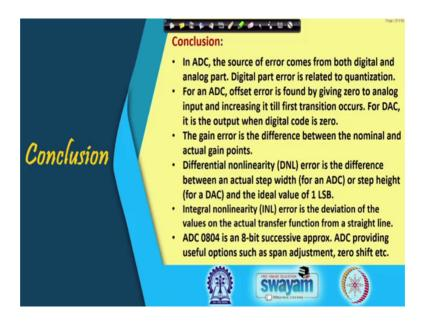
So, with this we conclude and what is we have seen that in ADC the source of error comes from both digital and analog part. And digital part error is related to quantization. And in ADC offset error is found by giving zero to analog input and increasing it till first transition occurs. For DAC, it is the output when digital code is zero ok. The gain error is the difference between the nominal and actual gain points. And we have seen it how it is calculated for both ADC and DAC.
