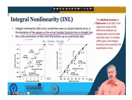
And from there, we go to something which is called integral non-linearity ok. And corresponding error is called INL error integral non-linearity error ok. And what is it, this is the division of the values on the actual transfer function from a straight line ok. And so let us see, how it is looks like, so this is the ADC right. So, this is the analog input value, and the corresponding digital code right.
