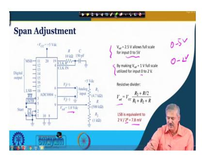
Now, what we discussed is the span adjustment ok. So, what is it, so let us see, so in this case here earlier it was 2.5 volt right, v reference was 2.5 volt. And the input voltage that was getting analog input voltage that was getting converted to digital equivalent was 0 to 5 volt right.
