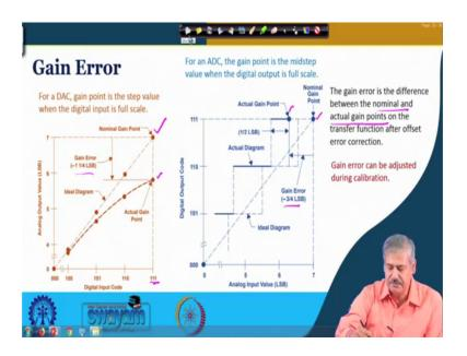
Now, next what we see is called gain error right. So, the gain error is the difference between the nominal and actual gain points on the transfer function after offset error corrections. So, after off offset error was there, so we have corrected by appropriate compensation right. And then you are finding out nominal and actual gain point.
