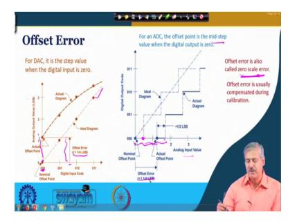
So, we begin with offset error ok. So, offset error is also called zero scale error ok, this is also known as zero scale error. What is it ok? So, for DAC as I said this part is common,
