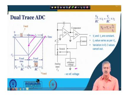
So, what people have thought off? In such a case that use of dual trace analog to digital converter ok. So, here what is happening you can see, that in the beginning so, if this is the circuit. So, this is the analog input voltage right now the first the ramp is generated this part, this is inviting so, the ramp will be in the negative direction right. So, this is the integrator op-amp that you can see have seen before so, this depending on this V X for a fixed time t 1, the ramp is generated.
