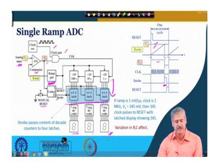
So, that we know in order limitation and how we can make use of it so, here is a single ramp ADC arrangement. So, initially these are the decade counters, this 3 are decade counters that you can see right. So, initially when you start so, it is it reset ok. So, these counters are already set you can see this reset signal going there ok.
