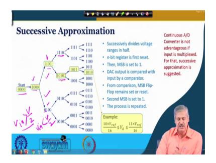
So, in the last plus when we ended, we discussed that continuous approximation, continues tracking type of ADC is good, but the problem with that is if multiple input is there; I mean, that need to be converted using a multiplexing kind of scheme, then it is not very suitable because it locks loses the tracking part of it and it is begin from the beginning which is not very advantages.
