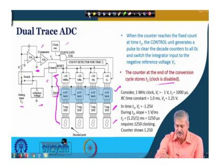
So, here if we look at the arrangement, the dual trace ADC circuit arrangement. So, certain things we can see which in the which is similar to you know single trace ADC, single slope ADC that we had seen before. So, this is the latch ok, this 7 segment display the 7 segment decoder driver, display, this is strobe of it so whenever this count as been completed.
