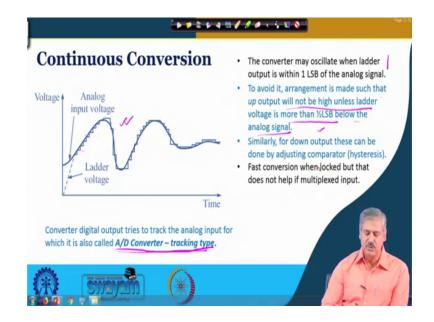
So, for continuous conversion so, this is what you would see happening for the input voltage and the analogue input voltage (Refer Time: 23:54) the ladder voltage, that is the digital to analogue conversion of the counter value, that is there. So, how they you know map each other. So, this is what you would see for a continuous type conversion ok.
