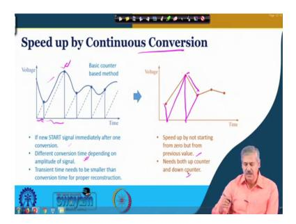
Now, in this counter based method, what we can see, that it is starting from here, if the new start signal comes immediately after one conversion of the analogue input voltage
