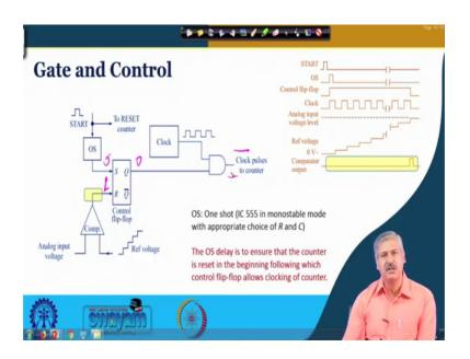
So, 1 and 0 now it becomes this becomes 1 and this is 0 it becomes reset right. So, this is reset means clocking is now stopped. So, at the output of the AND gate the clocking is stopped is it ok. And now whatever is the value that is the value related to the digitally coded value of the analogue input is it fine.
