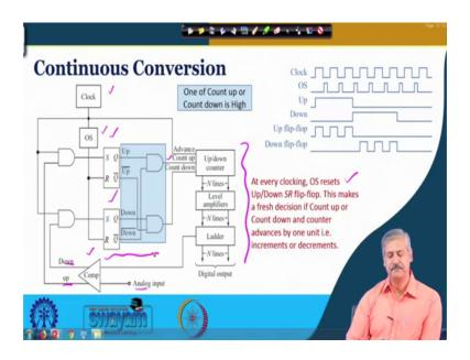
Now, for this we employ a circuit which is of this nature, which is a you know upgrade of the counter based circuit that we had seen before. So, we are already seen this block before ok, this block before right. Now, this is the comparator. So, depending on the value without this analogue input value is more or less right we are getting 0 or 1. So, we can convert it to up or down ok.
