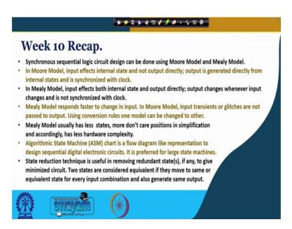
Very quickly what we saw in week 10 is how we use Mealy model and Moore model to design synchronous sequential logic circuit. And we had a comparison of these two different modeling techniques. So, in Moore model we had seen that input effects the internal state and output is generated from those states only. So, input does not directly go to the output logic generation.
