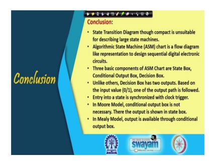
So, with this we come the conclusion of this particular class state transition diagram though compact is unsuitable for describing large state machine. This is what we have noticed ok. ASM chart is a flow diagram like representation which is useful for designing sequential digital electronic circuit to convert the problem statement to a particular chart which is easier for you know getting the circuit implemented.
