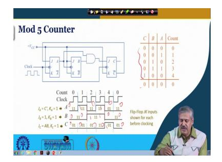
Now, let us look at mod-5 counter one arrangement, again there could be many different way, it can be made. So, there could be other than JK flip-flop other circuit as well right, even with the JK flip-flop there could be different arrangements. So, this is one arrangement ok.
