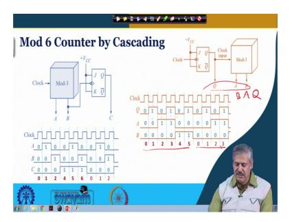
If that is the case, then let us see if we connect a mod-3 and mod-2, mod-2 you all know right 2, 4, 8, 16 right. So, mod-2 means only one flip-flop at its output, it is divided by 2 right, so that is mod-2 counter.
