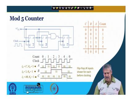
And before that, we also take a note that here C output is remaining at high for one clock period, in this particular arrangement ok. And so this can directly give you, this signalling that a count of 4 that is from 0 to 4 this has taken place 1 0 0 state has occurred right.
