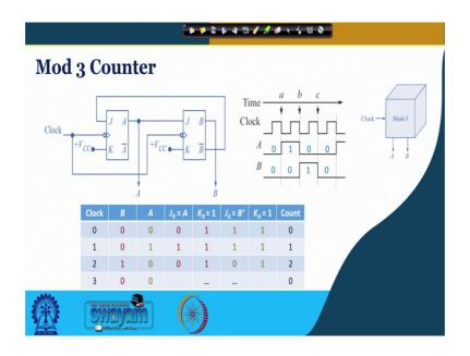
So, we begin with mod-3 counter ok. So, let us see the circuit of one mod-3 counter right, so it is made up of JK flip-flop right. And it is synchronous the clock is fed here right. And in this B bar is fed here as J input of A flip-flop ok. And A output is going as J input of B flip-flop all right. And K input for both the flip-flops are connected to logic high ok, very simple circuit the you can see all right.
