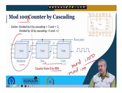
Finally, we can extend the way we were cascading in circuits to get higher modular number from 6 to 10. From now by connecting modulo 10 counter in cascade like this 7, 4, 9, 0 three of them, one after another ok. What we can get, we can get a modulo 100 sorry not 100, this is 1000 ok, please take a note of this modulo 1000 counter 0 to 999 ok, the count is possible right.
