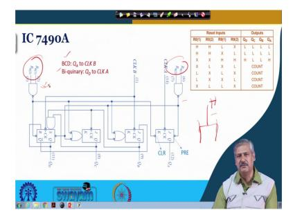
So, would like to see one IC 7490 ok, where we have a mod-10 counter implemented ok. So, IC 7490 A is one such IC right. And this IC has got a mod-5 counter over here right, and a mod-2 counter right. And you can see there are 2 clocks, this is one clock and this is another clock. This clock is associated with mod-2 counter and this clock is associated with mod-5 counter right.
