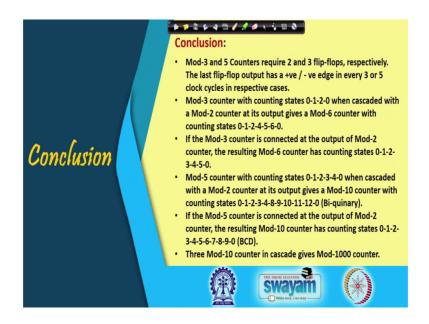
So, with this we conclude today's class, mod-3 and mod-5 counters we have seen required 2 and 3 flip-flops. And the way we have designed them is 0, 1, 2, 0, 4 mod-3 counter and when we have we are cascading it, we can get depending on whether mod-3 is there, before mod-2 or mod-2 is there, before mod-3, we can get 0-1-2-4-5-6-0 or 0-1-2-3-4-5-0.
