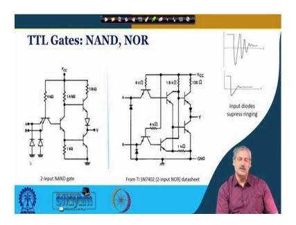
So, TTL NOR gate - if you look at the manufacturers specification. So, I have taken from a Texas instrument say, SN7402 technical document. So, what you will see here? These two input stages are in parallel and these two phase splitters are in parallel, and the totem pole part is common. And NAND gate of course, this is a multimeter NAND gate. So, this is how the TTL NAND gates and NOR gates are prepared, and the operation is known.
