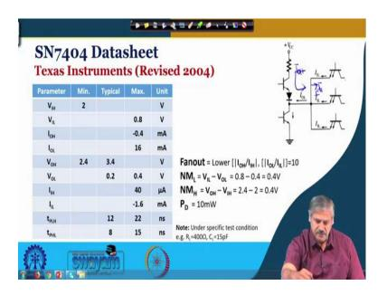
Now, we look at the - one practical, so I said that parameter was an estimated value. So, if you look at any standard manufacturers datasheet we shall see that how the TTL gate inverter 74 say, 04, what are the different parameters how that is been specified, ok.
