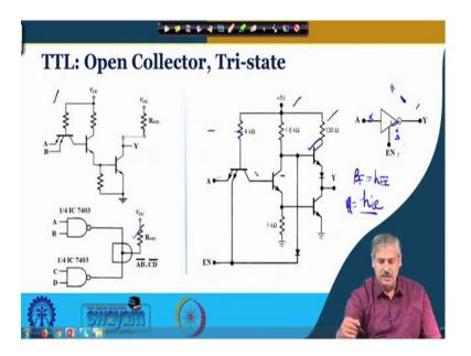
Now, TTL open collector - how does it work? So, in the TTL open collector, the last stage in the totem pole you do not have any resistance, ok. So, this remains open. So, to make it work we need to connect an external resistance to it, ok. So, this is the external resistance through it. So, this is called pull-up resistance also, ok.
