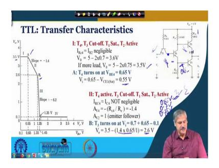
In the last class we got introduced to TTL, and there we ended by saying that a phase splitter - this is the phase splitter that we see is important when we talk about the TTL, when we talk about TTL activity, and the totem pole output configuration. So, this is what, how we ended in the last class.
