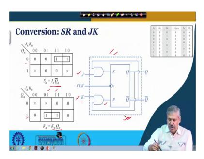
So, now to have a minimized expression for this right; so, we can see that one group is required here, so that is coming as J n remaining constant with value 1, and Q n with value 0, so J n Q n bar. So, as an we can simply write it this way, because we need to cover only the once that is the largest group possible. And for R n, we can see that it is K n remaining value with 1 and Q n with value 1, so it is K n Q n ok.
