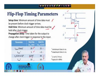
To end this particular lecture, we just would like to get you know introduced to another important concept is that of flip-flop timing parameters its significance ok. So, as I said the timing diagram is the key to exhibit how the things happen workout with respect to time, which is not very clear from the truth table, excitation table or other form of you know representation. So, we take help of this timing diagram to discuss to understand the
