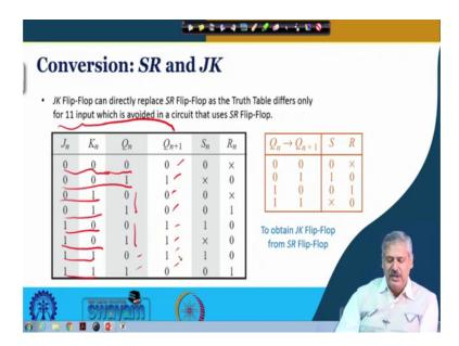
Now, let us look at another example ok, where we have JK flip-flop required from SR flip-flop ok. So, given a SR flip-flop two you know two input and we require a JK flip-flop. We can do it for any other type that is one type to another, so let us look at this one
