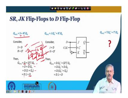
Now, if we are looking at converting other flip-flop to D flip-flop right. So, if we are looking at SR flip-flop getting converted to D, we have seen before. Otherwise, also we can figure it out from their equations the characteristic equation. This is Q n plus 1 is equal to S plus R prime Q n. And if we consider S as D, and R as D prime which we are done before, but we can put it in the characteristic equation.
