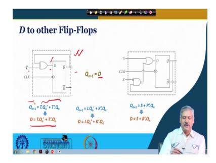
So, simply we can write D as T Q n prime plus T prime Q n ok. And that in the logic circuit this is a computer logic circuit right, so we can get by designing it. So, this is your T input, and this is just an XOR ring. So, basically Q and Q and getting XOR, and it is being available here as D input. And when the clock trigger comes, whatever is here it will go there ok. So, whatever is here that is this will go there. So, this is very simple for converting D flip-flop to T flip-flop ok.
