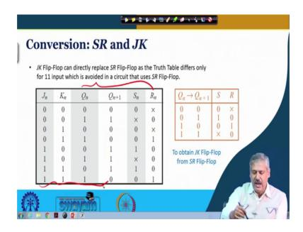
So, we can now understand that this part is the SR flip-flop excitation table, which is deciding the entries right. And these part JK flip-flop truth table are deciding the entries. So, this is this JK flip-flop truth table itself is it ok. Now, with this table in hand ok, we now move to next step.
