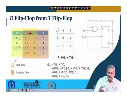
So, let us look at this problem of getting a D flip-flop out of T through a synthesis example, you know synthesis of logic circuit example not going through a algebraic
