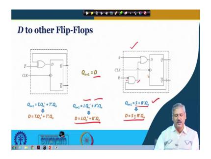
So, this can be extended to JK flip-flop as well. So, JK flip-flop equation is similar, but it is J Q n prime plus K (Refer Time: 04:13) prime Q n ok. So, we will take D as this one ok, and then we shall just make it combinatorial circuit, and accordingly we will get it right. And similarly, for D flip-flop getting converted to SR flip-flop ok. So, the equation is Q n plus 1 is S plus R prime Q n. So, we can write S as D as S plus plus is here or we know that, so R prime Q n ok.
