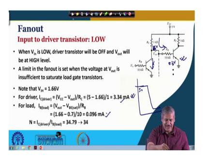
But there may be an issue when the input to the driver is low. So, this is the input to the driver when it is low the output is high, you have, you have already seen right; the characteristics part of it - isn't it? So, the characteristic show us like this. So, when input is low the output is high; so this particular thing - right. So, this output high we are connecting to many such gates - right and, whenever it is connecting these are drawing base current - right.
