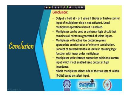
So, with this we complete the depletion on multiplexer very quickly what you have seen that output is held at high or low depending on output is inverted non inverted by when the strobe enabled control input of the multiplexer chip is naught not activated and when it is activated normal multiplexing operation takes place multiplexer can be used as universal logic circuit ok.
