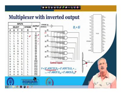
So, if this is clear. So, we look at another circuit multiplexer circuit which is there where the output is inverted earlier we have seen all the output is just you know whatever is the input output is following the input ok.
