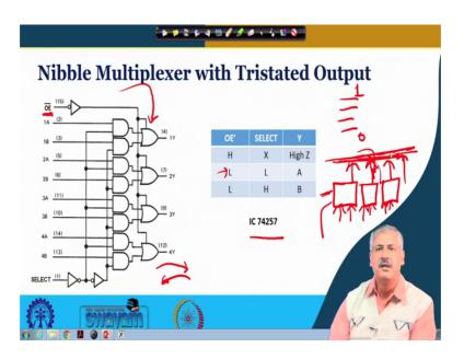
So, now, at times this nibble multiplexer is connected in a manner where many such units are trying to place data. So, this is one block, this is one nibble multiplexer, this is another nibble multiplexer right and they are trying to place data over a common line depending on which one is getting selected.
