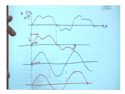
If somebody says I have a flux density distribution which is quite arbitrary like this, I mean how one will get it that is besides the point the, but the point to be understood is this is flux density along space, suppose it is distributed along x axis in this way and beneath it I am moving a conductor in this way. So, if this is the b distribution, b which I will write now small b because I find it is not constant at all the points, but it is repeating
