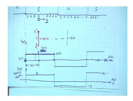
Suppose you have a certain portion of space, South Pole, North Pole South Pole; that means, lines of forces are doing like this here and suppose this field are constant value and it is doing like this and so on, and then doing like this. And it is conductor is here with its x 1 y 1 terminal, I am looking from the top. So, x 1 y 1 can be seen and then applying right hand rule I know this is plus, this is minus ok.
