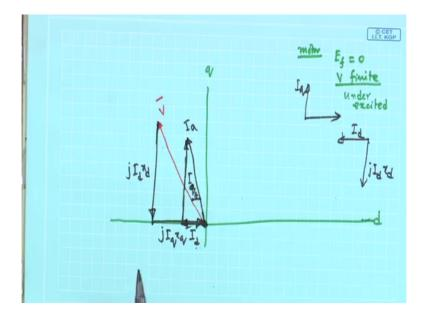
I will edit drawing nicely. See the it is motor mode, so what you do with excitation 0 ok. So, I draw q-axis, please let me be with me, so this is d-axis. And your field current will be 0, it will be somewhere and it is definitely E f equal to 0, and V finite; V finite and it is motor mode. These are the informations you need motor mode. So, the machine is under excited under excited, under excited synchronous motor always draws lagging current ok, it will draw lagging current.
