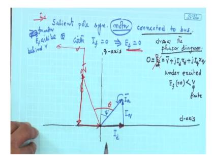
Now, similarly let us draw the phasor diagram of a salient pole synchronous motor connected to bus, and field current brought to 0 ok. So, salient pole synchronous motor, now it is operating in motor mode connected to bus with I f equal to 0, which implies that E f is equal to 0 is not, so this is the situation.
