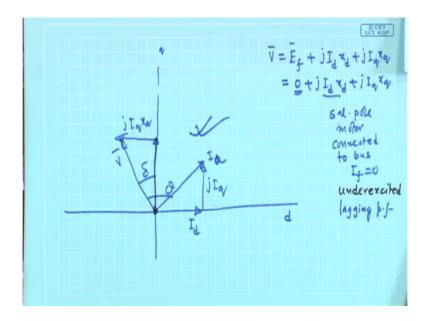
So, this synchronous motor with field current 0, we were discussing. And the interesting, thing I would like to tell about the drawing of the phasor diagram which very quickly let me do it, so that we can see this is q, this is d. But, in case of motor I was telling that I will start with E f, this was the thing you must be very careful about I a plus j I d x d plus j I q x q most probably, while adding I started with E f, and that is the confusion.
