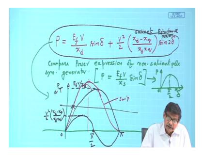
Recall that so, we have got the power as E f V by x d sin delta minus V square not minus plus; this is can be written also in this form x d minus x q by x q by x d x d x q into sin 2 delta. This compare it, compare power expression power or torque this is synonymous
