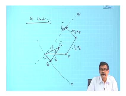
So, leading generator leading: so, a typical thing will be this is V your E f will be above it ok. So, suppose this will be E f q axis, this will be your d axis and this is 90 degree and then this is suppose your I a. Then what I have to do? Then you know this angle is delta, this angle is theta. Then I a I have to break it up into two components d axis that is I d and this is I q.
