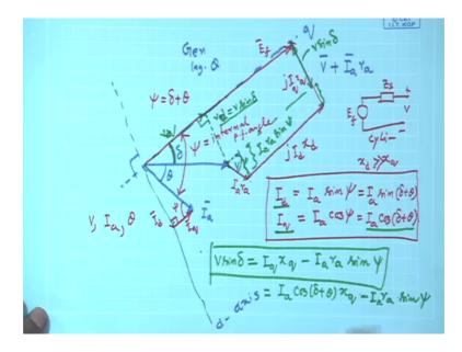
And I have taken Generator mode of operation and it is supplying lagging power factor angle theta and I told you how to do it.
