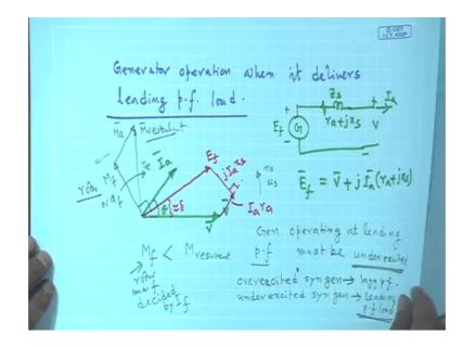
Now, suppose I will just draw for generator operation, I will draw the phasor diagram. Generator operation when it delivers when it delivers leading power factor load; leading power factor load it will be like this. So, how I am drawing generator plus, minus, here is the E f, here is your Z s. I will now draw for this whole thing Z s. This is r a plus jx s and this is your terminal per phase voltage V and I am saying it is delivering a leading current.
