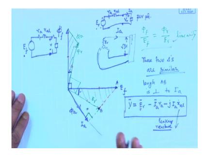
Therefore, we say that this is your phi f under no load condition open circuit condition, this is your Ef fine. And this is 90 degree. Now you load the machine suppose this is your I a.
