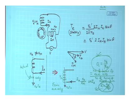
And we have shown you that in a single phase induction motor, there is a rotor like this cage rotor and there will be a main and auxiliary winding.
