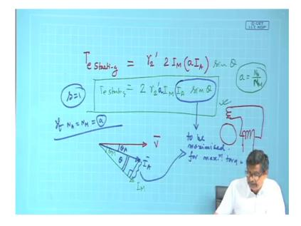
If that be the case then this expression of starting torque that is T e starting will be this r 2 dashed into 2 I M, but this auxiliary current I will write a I A into sin theta where a is N A by N M. In synchronous what that is that will be the expression of the torque starting torque. Or this is equal to 2 r 2 dashed r m s value of main winding current r m s value of actual auxiliary winding current and sin theta.
