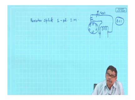
Now what happens is this now suppose let us try to understand resistors split how to chose optimum value resistors split single phase induction motor. That is the goal will be it can be shown like this auxiliary winding. I will connect some r external. All things are happening at a s equal to 1.
