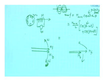
Suppose this machine only I am considering this is the rotor this a point to be noted what I am telling, single winding thats all. Here is V bar M and I now know and also explained that if you excite this at starting no torque machine will never start up, but if it is already rotating n r, it will continue to run that is what the conclusion was.
