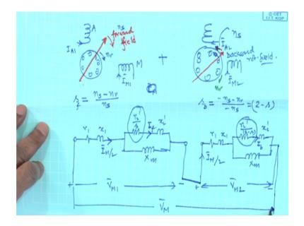
These two motors are at work, balanced 2 phase motor balanced 2 phase motor. I mean go back to that primary thing and it is a balanced 2 phase motor, its torque slip characteristics will be same as that of a 3 phase induction motor. Similarly this is another balanced 2 phase induction motor. Its torque slip characteristics why it will be other than we what we obtained for 3 phase induction motor; same. So because each one of them is a balanced 2 phase induction motor in this case.
