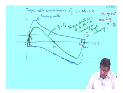
Therefore, torque slip characteristics of single phase induction motor will be like this. Suppose approximately this is s equal to 1, this is s equal to 2, suppose for the forward motor, the torque slip characteristics will be just like that of a single phase induction, a 3 phase induction motor and slip I have varied from 0 to 2. Why it is varied from 0 to 2, you will easily understand.
