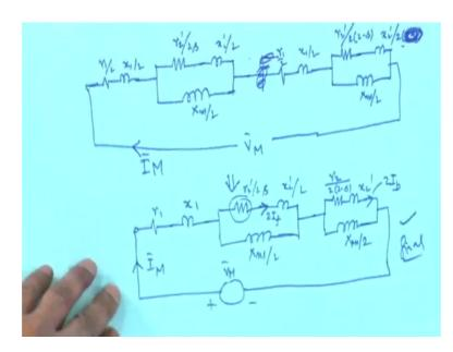
So, divide all the impedances by a factor of 2 and redraw the circuit that is I will do very quickly x 1 by 2, but this is a very important stage and then I will make it r 2 dashed by 2 s, all impedances I will divide by 2, x 2 dashed by 2 this is magnetizing inductance X m by 2 and then once again that backward motor it is connected in series oh. So, there will be another r 1 by 2, another x 1 by 2 and this two parallel branches that is r 2 dashed by 2 into 2 minus s that is what I am doing.
