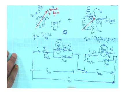
Let this induction motor whose rotor is this whose rotor is this and suppose the rotor is moving at some speed n r and this is your main winding and this is the assumed auxiliary winding having no current.
