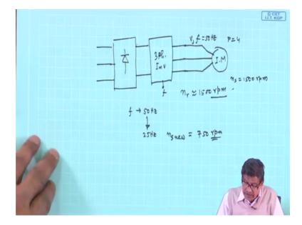
I will give you simple idea see suppose you have got this supply, your three-phase supply rectifier and DC and three-phase inverter. And I told you can both vary the magnitude of the rms voltage and frequency that is v by v and f can be varied depending upon requirements you do it like that and here is your motor and it is supplied, induction motor.
