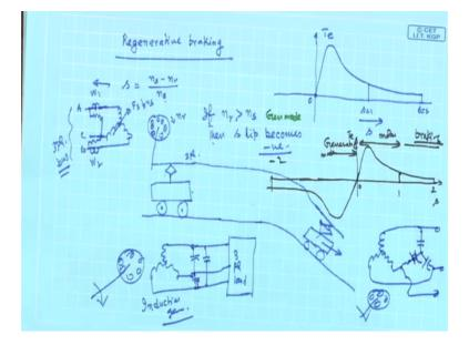
I will just tell you the ideas here; no question of going that ok, this was the motor if sum of the speed become greater than n s then generator mode; generator mode it goes. Then it looks like this top slip characteristics whatever I am drawing, it will be like this from s equal to 0 to s equal to 2. Between 1 and 2, it will be some braking mode it has gone.
