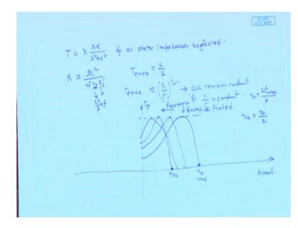
Just to get a firsthand experience how the speed will change. So, we know this is the expression of the torque if all stator impedance is neglected all stator impedance is neglected and mind you what is the value of K. K was some 3 V 1 square by 4 pi n s most probably like this x 2 dash K the constant value and also we noted that T e max T e max was equal to k by 2 now. So, this was the thing most probably T e max
