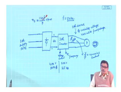
Suppose, rated voltage is 400 volt 50 Hertz actual machine rating I suppose decide I will run it at 400 volt because inverters gives you variable voltage variable frequency I will adjust it to 400 volt and 25 volts I want to run it at half the rated speed. Suppose, what depending suppose p equal to 4 rated speed is 1500 rpm, 50 Hertz supply.
