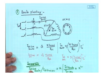
Only thing I leave it to you to try to understand even if it is wound-rotor induction motor you could apply it; I mean no problem if it is wound-rotor induction motor rotor shorted you could adopt any of these method, but since wound-rotor motor that facility is there you can do like this, similarly auto transformer starting.
