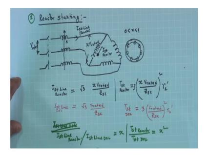
And, you remember that if we use reactor starting your starting current will be reduced only by a factor of x I am not writing that and starting torque will be reduced by a factor of x square and I am comparing these with respect to direct on line start, ok. (Refer Slide Time: 00:52)
