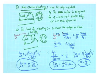
Number 4 star-delta method of starting three-phase induction motor; in this case and this can be this you now note down can be only applied if the stator if the motor is designed for delta connected stator winding; stator winding for delta connected stator winding for normal operation, that must be understood.
