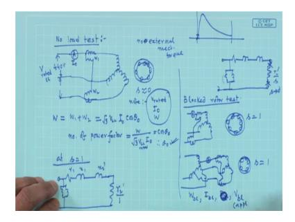
First let us come to no load test. In no load test, suppose this is the motor let us assume it to be star connected, and the rotor may be cage or rotor suppose cage this is the rotor here is your supply. So, under no load condition, you apply the full rated voltage that is 440 volt here line-to-line, V rated you apply line-to-line and give supply to this, and record the ammeter reading. And connect better 2 watt meters and W 1 plus W 2 gives you the total input power.
