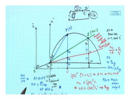
So, suppose this is your v 1 the supply voltage whether, this is your v 1. First of all v dash equal to 0, that r 2 by S is open current drawn is only I naught that is the no load current. Suppose that is I naught and I naught plus I 2 dashed voltage applied to this parallel branch, to this branch is also v 1. So, this current tip of this current facer I 2 dashed it will lie on the perimeter of the circle.
