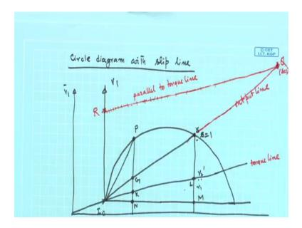
So, circle diagram with slip line. So, what is the thing? This is the thing this is supply voltage v 1, this is your no load current I naught and here is that parallel branch where r 2 pi s stays I will draw a bigger one and this is the circle, any point I 2 dashed this current will be I 2 dashed ok.
