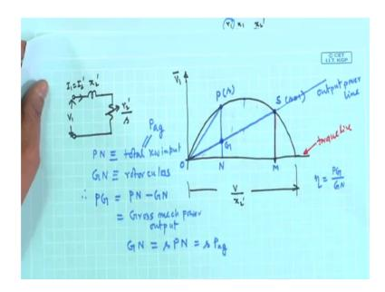
Because this is the air gap power so from whichever line you record this air gap power is called the torque line, but here it is tilted because of the stator copper loss and therefore, you can if you divide this SM length in the ratio stator resistance is to rotor resistance reflected values join these points for any operating point it will intersect that SK, then KN also represents the stator copper loss this intercepts will all represent stator copper loss.
