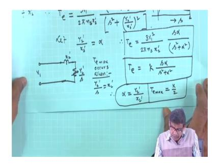
So, with that in mind we have got this. And here once again you see, the value of T e max maximum value of the torque will be for x write alpha if you do that, it will be k by 2. So, these are the three things, maximum torque is this k divided by 2.
