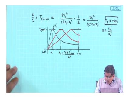
And what is the expression of T e max; let us write that T e max in terms of equivalence circuit parameter. In this case, it is only r 2 dashed and x 2 dashed, it will be 3 V 1 square by 2 pi n s into x 2 dashed that is this k into half, because s equal to alpha, it gives you
