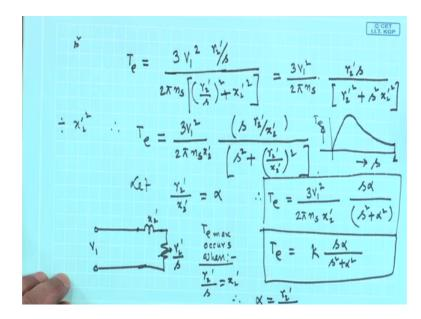
So, we proceed from this, therefore once I 2 dash is known, then I substitute this I 2 dashed here. So, to get the torque developed by the machine as T e is equal to 3 I 2 dash square that is V 1 square by r 2 dashed by s whole square plus x 2 dashed square. And by 2 pi n s is there into in the numerator r 2 dashed by s, this is the expression of the torque developed by the machine [FL].
