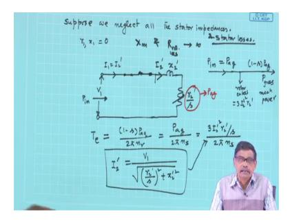
Welcome. So, we were discussing about somewhat simplified equivalent circuit of 3phase induction motor, which are very much used I mean and so that you can quickly get the idea about the performance of the induction motor. So, what I told is that you find out the equivalent circuit.
