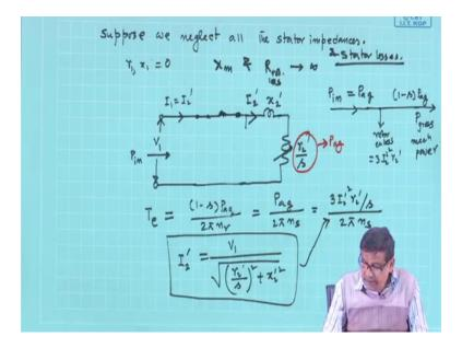
Suppose, we say that suppose we neglect all the stator impedances, what do I mean by this? That  $r 1 \ge 0$ , it is stator you neglect them x = x = 1 and this rotational resistance, this is neglected means what? These are pretty high I mean you must understand.
