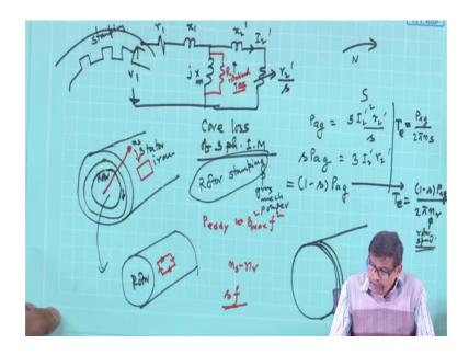
Now, therefore, when I draw the equivalent circuit of a three phase induction motor, whether same equivalent circuit will be valid, I will say yes, it will be. This is  $r \ 1 \ x \ 1$  and this is your x m and this is your x 2 dashed and r 2 dashed. That is how I was drawing at least for a slip ring induction motor. This is my supply voltage, is not, I was drawing at any slip. Now, the question is if it is a cage type induction motor whether can I draw this type of equivalent circuit?
