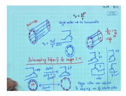
In nowadays, the thing is that do not touch p. I mean, what is the point of having another winding synchronous speed of the induction motor then can be changed 2 f by p. So, supply frequency I will vary p, I will not touch cage induction motor or slip ring induction motor I do not care, p I will not touch, supply frequency I will vary. We will discuss about these things a little later, but this is the things I wanted to tell about the cage induction motor.
