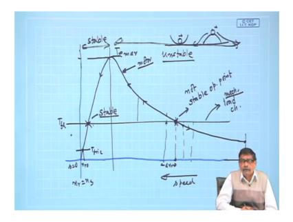
So, it is suppose the torque slip characteristics make practice drawing yourself. So suppose this is the, a typical well designed 3 phase induction motor the torque slip characteristics is like this. This is once again s equal to 1 this is s equal to 0 this is T e max. Although here also I have not drawn properly this should be one-tenth of this approximately I mean this is T e max. [FL].
