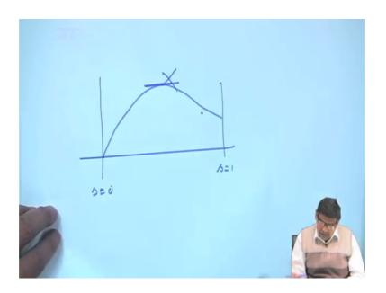
Correctly means do not draw a torque slip characteristics of a well designed induction motor; something like this s equal to 1 s equal to 0, students are often found that they draw it like this; and no never draw. Because the T e max for a well designed motor will be closed by s equal to 0 a typical value I told it is s equal to 0.1.
