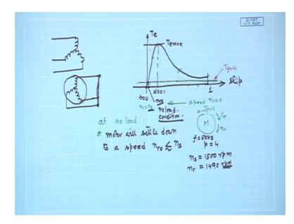
Welcome and so we were discussing about the Torque Slip Characteristics of a 3 phase induction motor. And which is very important, it gives us an opportunity to understand how the machine settles down to a particular operating point. And under no load condition I told you it will be like this.
