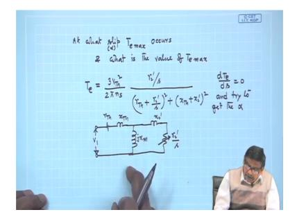
Then the next question comes in terms of equivalent circuit parameters can we tell what will be the value of T max and at what slip that T max occurs. So, so at what slip T e max occurs, and what is the value of T e max can we derive some formula, what is the value of x T e max.
