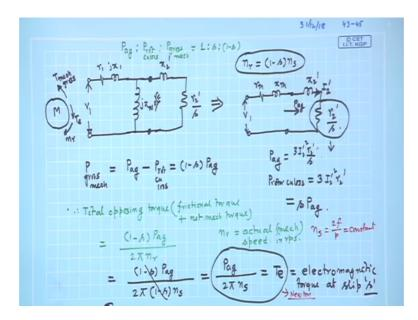
So, I we develop this equivalent circuit and told you that this is the equivalent circuit which is a stator resistance stator leakage reactance per phase. Now, it is similar to that of a transformer, and then you have this magnetizing branch which is  $j \ge m$ . I mean all reactance's are j that is there.
