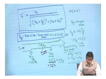
So, the input power to this circuit is and I drew this I will not waste time. Last time we told you that this equivalent circuit means, you are giving some input power drawn from the supply out of which a portion will be lost in the stator coils, as stator copper loss 3 I 2 square r Thevenins that is value will be I mean I 2 dashed squared r Thevenins.
