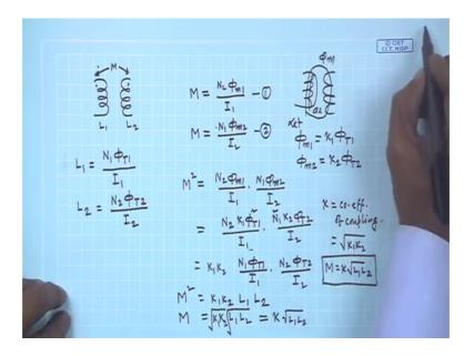
These are the 2 coils having inductances L 1 L 2 and this is the mutual inductance M. And we know that M is equal to say M is equal to I can write as N 2 phi m 1 by I 1 and this M is also same as N 1 phi m 2 by I 2 when the first coil is carrying some current flux linkage per unit ampere and so on.
