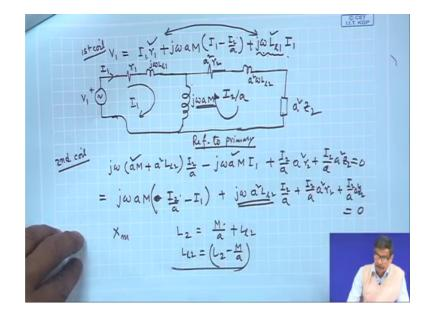
And is it not the same equivalent circuit we got from physical considerations of a transformer? See r 1 and this is leakage reactance this is the mutual inductance which we denote by X m. But in terms of M it is a into a M where a is the number of turns ratios N 1 by N 2 and all the impedances on the secondary side is reflected as a square into r 2 a square into omega 1 2 and so, on a square into Z 2.
