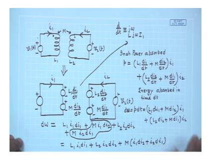
So, we take in the same way these two coils; suppose these are the dots and here I will connect 1 source and let us assume this coils has got negligible resistance almost ideal coil. So, here you connect a source v 1 t and current absorbed by this coil is i 1 similarly you imagine you have connected another source v 2 t here and its current direction is like this.
