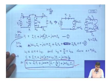
And finally we wrote down the KVL equations from the two sides remembering the fact how to put the dots on these two coils knowing those dots I will be correctly writing the KVL equations with the appropriate polarities of this voltages students often make confusion
