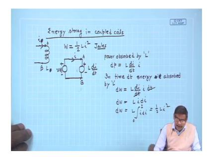
It will take few steps energy storage in coupled coils. The thing is if we have a single coil and it has got self inductance L 1 and this is suppose you are passing some current I 1 through it I because no point in taking telling about L 1 L 2.
