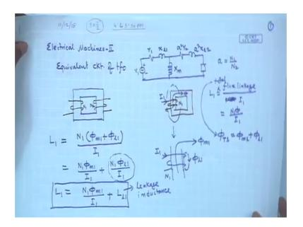
That we tried to found out the equivalent circuit of a transformer from circuit point of view and from the concept of a self and mutual inductances you recall very quickly I will tell that. So, this is 2 coupled coils having turns N 1 and N 2 and then when you pass some current through the coil it produces flux the direction of the flux can be obtained by wrapping your other fingers along the flow of the current and thumb will give you the direction of the flux so, phi.
