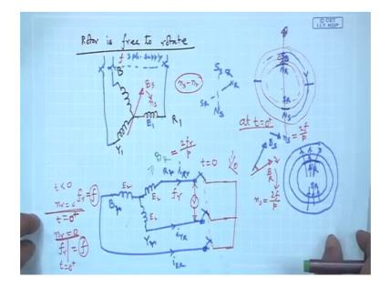
And in our last class, we came up to this that is you recall that at t equal to 0 we first observed what is going to happen and we told you that frequency of the rotor current are one and the same. Rotor is yet to rotate, but it is carrying current at t equal to 0 plus it still remains 0 because of its inertia and rotor frequency at 0 plus is p by 2 into n s minus n r which is p n s by 2 and then, it is supply frequency f.
