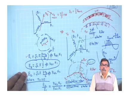
For example, what I am trying to tell that in this expression flux per pole phi what should be used because in this stator coil e1 root 2 pi p n s by 2. Both of them are moving no doubt with synchronous speed. This term remains same, but what is flux per pole? Which flux per pole should I use? Understood this is the issues and this can be very nicely explained and this will come slightly later.
