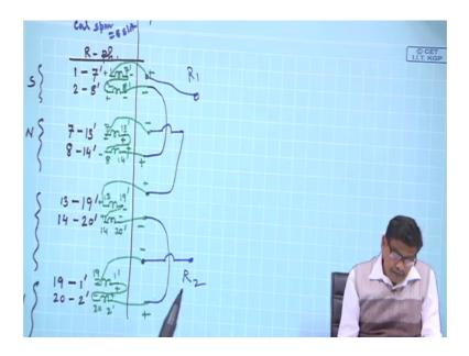
Welcome to this next lecture on Electrical Machines and we were discussing about how to make a balance 3 Phase Winding, when this specifications are that total number of slots is 24 and number of poles is 4, this time I have taken that is that is this was the specification 24 slots and 4 poles machine double layer winding I want to do full pitched and I have decided that under each pole there are 6 slots 2 slots will be allotted to R phase for distribution.
