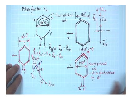
Which is denoted by this symbol K p p stands for pitch factor. Now what is a pitch factor? Pitch factor is this I told you for any coil like this multiple turns are there this is the coil turn terminal. So, when these are joint means this it goes several times.
