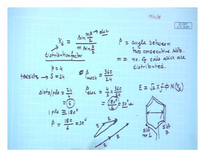
If I write the formula straight away it was like this sin m beta by 2 divided by m sin beta by 2. What is m? What is beta? Beta is the angle between 2 consecutive slots angle between 2 consecutive slots in electrical degree and m is the number of coils number of coils which are distributed which are distributed so this is very important. Therefore, I will now first tell you how to or what does this mean actually.
