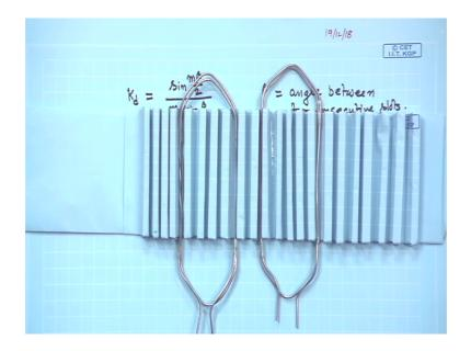
It means that if you have the slots here and if you have suppose 2 coils this 2 coils each one of them is having 2 times here 2 turns you can easily see and you could make them accommodate in one slots only a pair of slots only and then you connect this 2 coils in series here. Therefore, total number of turns will now become 4 as if it is a multi turn coil with 4 turns.
