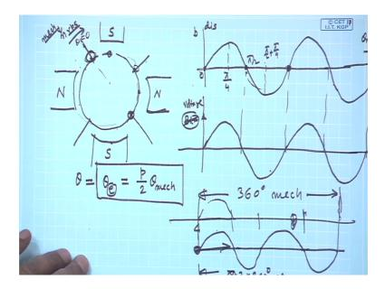
Now, let us see what happens, if it is a four-pole machine, suppose I will first draw the rotor, otherwise I am sketching the rotor so badly. So, this is the thing. Suppose, this is South Pole, we know how to create a four-pole structure. By not using projected poles only; by passing some current through the coils housed in stator ok, those I am not repeating. So, suppose effectively, it comes to this some South, North, South, North.
