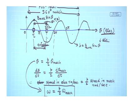
Suppose, I will say that this is a four-pole; four-pole machine 1, 2, 3, 4, this is 360 degree mechanical no doubt. But, in electrical angle if theta is in electrical that is how I should describe its sine wave, so that it will fit in, I will write it as B max sin theta and this theta as I told without any suffix means electrical angle, so B max sin theta.
