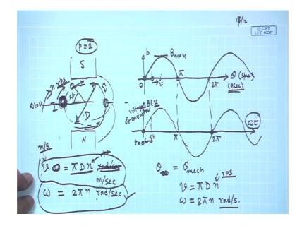
The whole idea is this that if it is a two-pole machine, your b distribution if it is sinusoidal. The fundamental component of that b distribution only we will consider, we will see that how this can be made more perfect a sinusoidal b distribution. But, assuming that b distribution is this a conductor if it is moving underneath this b distribution, then the induced voltage across it will be just same as this b distribution.
