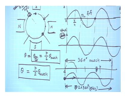
So, this is very important. Electrical angle is equal to p by 2 theta mechanical and one should not forget. If it is a six-pole machine, it will be 3 times the mechanical. Three cycles of EMF will be generated, when the conductor moves mechanical angle of 360 degree round. So, this is the very important thing. Therefore, it looks like that it is necessary to distinguish between electrical and mechanical angle, space angle, so what we will do is this?
