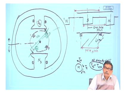
I will draw it somewhat slightly in nicer way; suppose this is the every rotating machine is having some stator and rotor. And this is the stator iron with this cylindrical and there may be coils wrapped around the poles and later we will see there are several other possibilities. But, just and if you pass this current like this, this becomes a north pole of the stator because lines of force will come out and this will become south pole of the stator.
