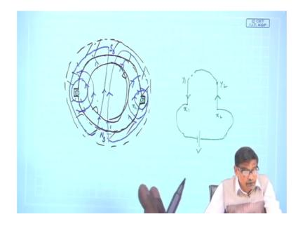
For example you can now think that stator I have till now shown some projected poles, but I can make a stator like this. Totally cylindrical, annular I mean, these are iron and it has got a length perpendicular to the paper and it goes around, so iron made of iron. Now I can, I had instead of projected poles like this, I can touch slots here and here is another slot, so this is the stator. Now only a pair of slots, the there is nothing here, it is open, a groove.
