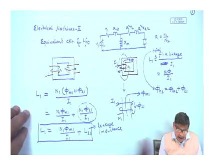
Therefore the course begins with electrical machines II and as I told you equivalent circuit is one of them. So, let us not leave a transformer in its totality. Because the equivalent circuit of the transformer you must be remembering, we will start from that; assuming you have undergone a transformer course, but I will try to arrive at the equivalent circuit of a transformer in a from the viewpoint of circuit analysis.
